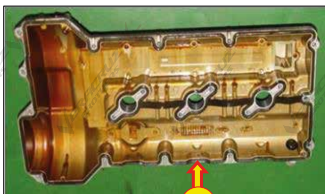
Gasket Installing Groove (Cleaning area)
