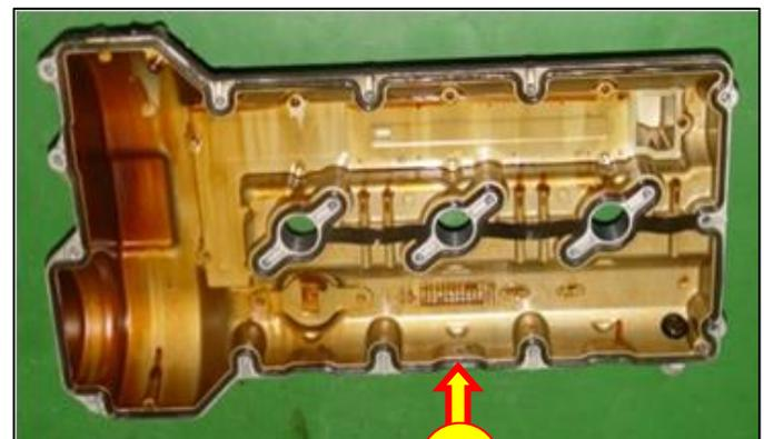
Gasket Installing Groove (Cleaning area)
